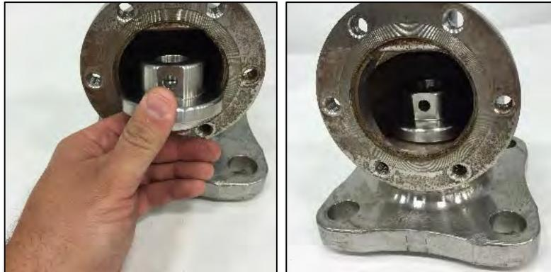
*Figures 5.6 and 5.7 Seal Disc in Valve Body*
