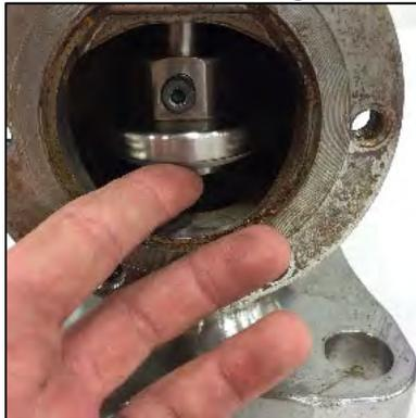
*Figure 5.12 Seal Disc Installation*
