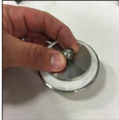
*Figure 5.5 Seal Retainer Installation*
