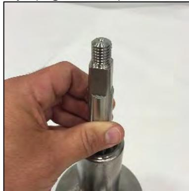
*Figure 3.15 Valve Stem Removal*
