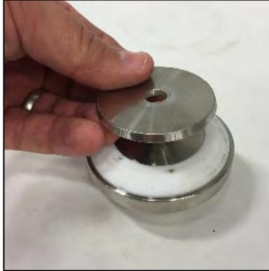
*Figure 3.20 Seal Retainer Removal*
