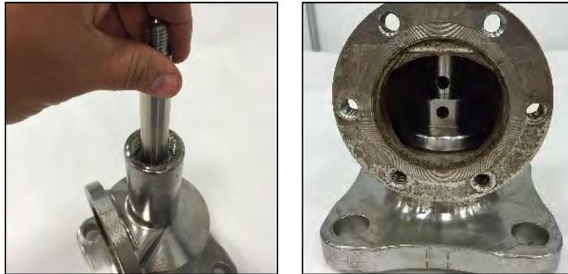
*Figures 5.10 and 5.11 Stem into Valve Body*
