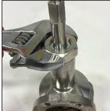
*Figure 3.11 Jam Nut Removal*
