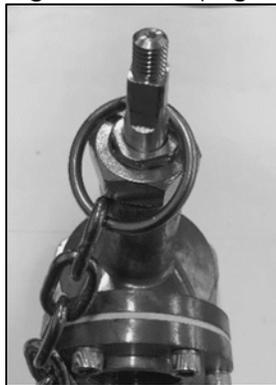
*Figure 6.2 Plug Chain Ring on Stem*
