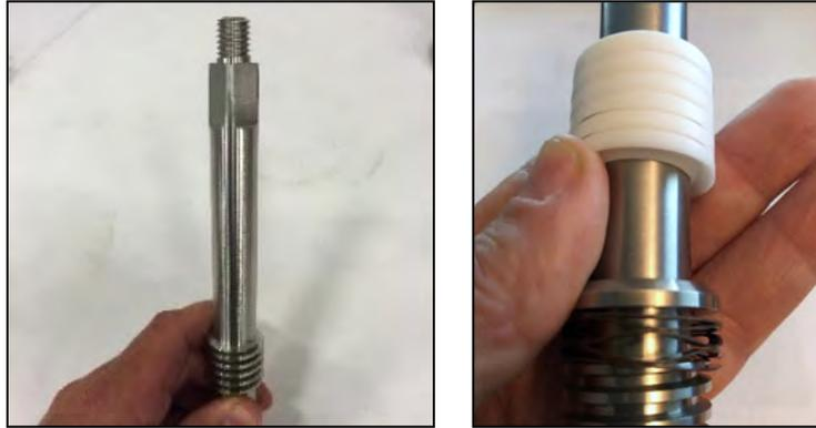
*Figures 5.8 and 5.9 Packing Kit onto Stem*
