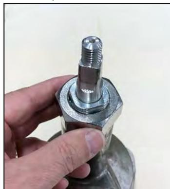
*Figure 5.15 Packing Screw Installation*
