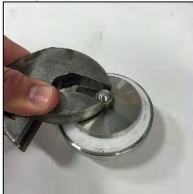
*Figure 3.19 Disassemble Seal Disc*
