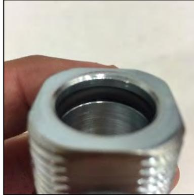
*Figure 5.13 O-Ring Installed into Packing Screw*
