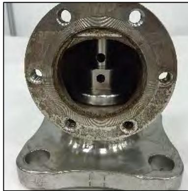
*Figures 3.5, 3.6 and 3.7 Seal Disc Removal*
