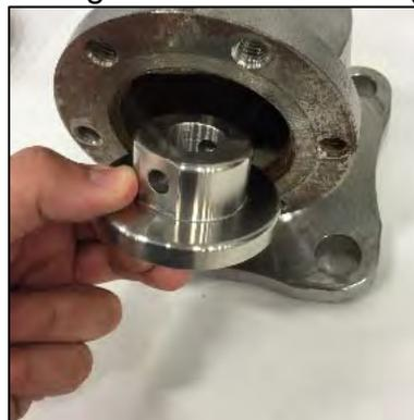
*Figure 3.8 Seal Disc Removed*
