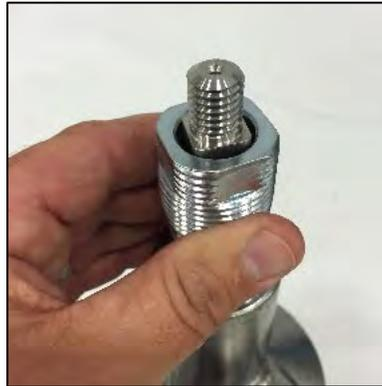
*Figure 5.14 Packing Screw into Valve Body*
