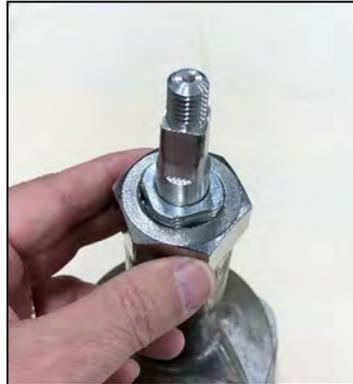
*Figure 6.1 Torque Packing Screw*
