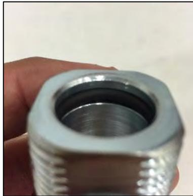
*Figures 3.12, 3.13 and 3.14 Packing Screw / O-Ring Removal*
